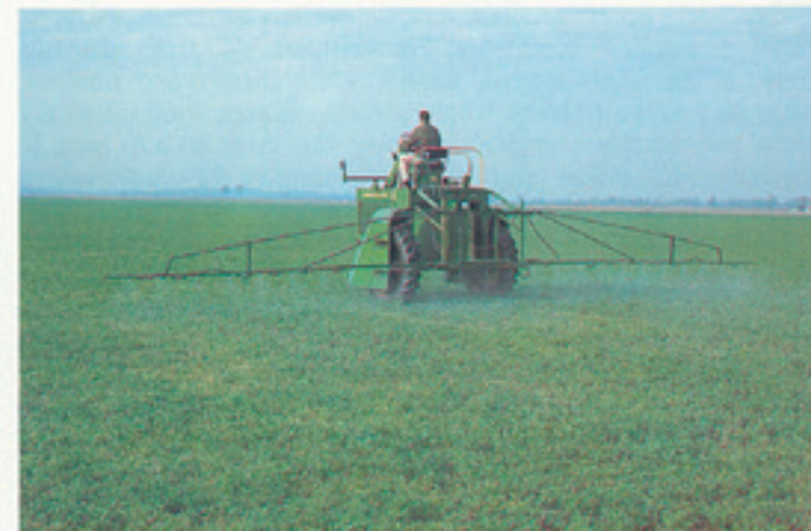
Above: Correct adjustment of sprayer boom for coverage and penetration of the foliage is necessary for alfalfa weevil control. The most satisfactory results are obtained with a spray volume of 20 gallons per acre.
